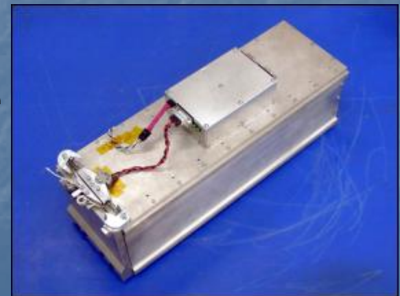
Canada's XPOD Triple Launch Tube
